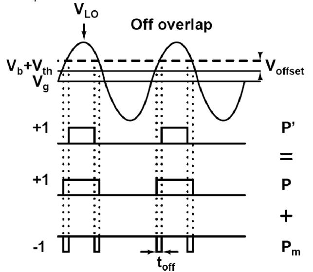
Fig. 5. The effect of switch bias on IIP2 for passive mixer.
