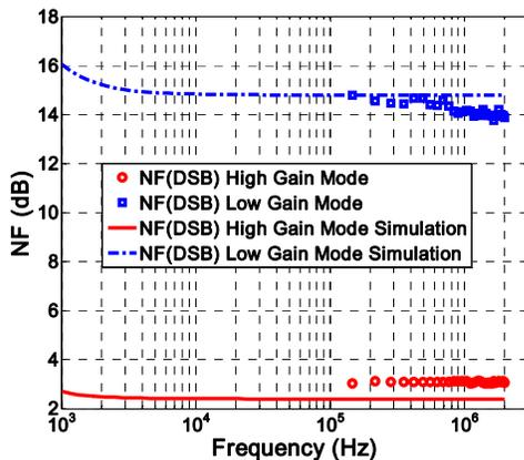
Fig. 7.  $NF(DSB)$  for High Gain Mode and Low Gain Mode.
