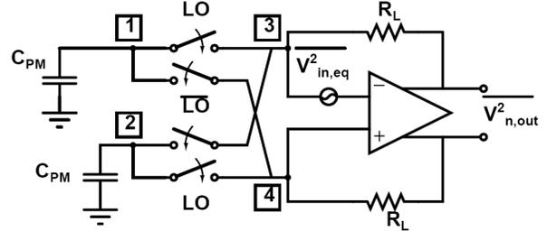
Fig. 4. Transfer of the noise from baseband amplifier to the output through the switched-capacitor input resistance.
