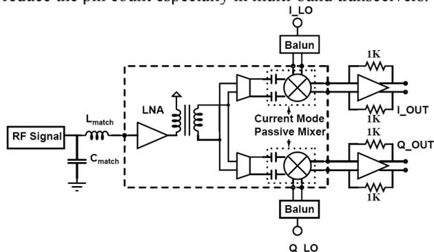
Fig. 1. Block diagram of the front-end.
