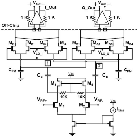
Fig. 3. Balanced transconductor driving the current-mode double-balanced passive CMOS mixer.
