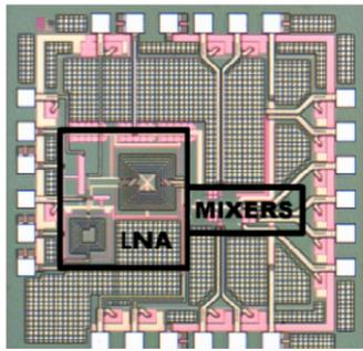
Fig. 6. Die photo of the front-end prototype.
