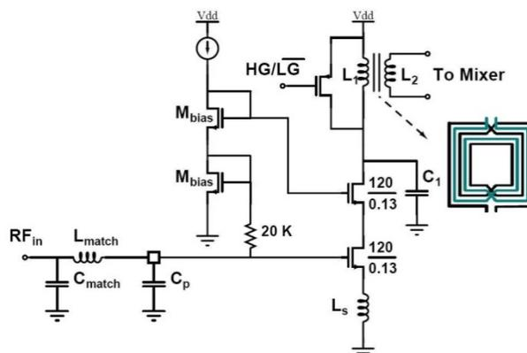
Fig. 2. LNA with on-chip transformer load.
